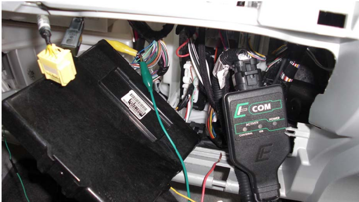
Figure 22. Ecom cable spliced directly into the Power Management ECU.
