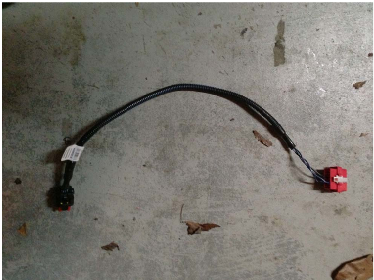
Figure 11: Handmade ECOM-OB2-II connector
