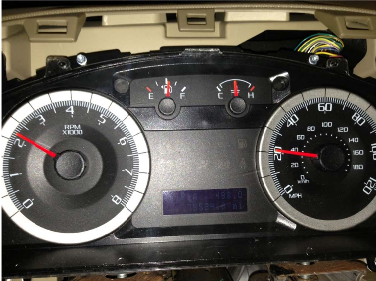
Figure 18: Manipulated RPM and speed readout.
