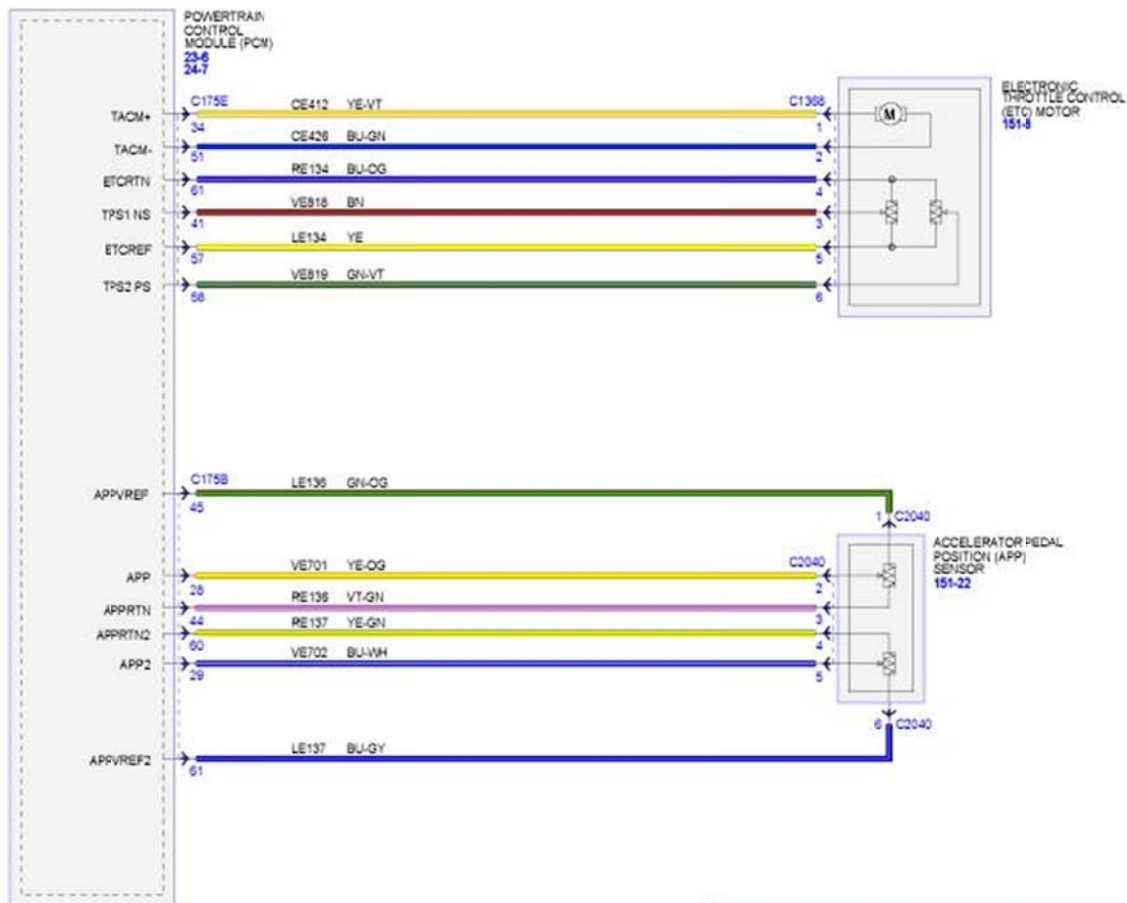
Figure 15: The electronic throttle control and accelerator pedal position sensor are wired into the PCM.
