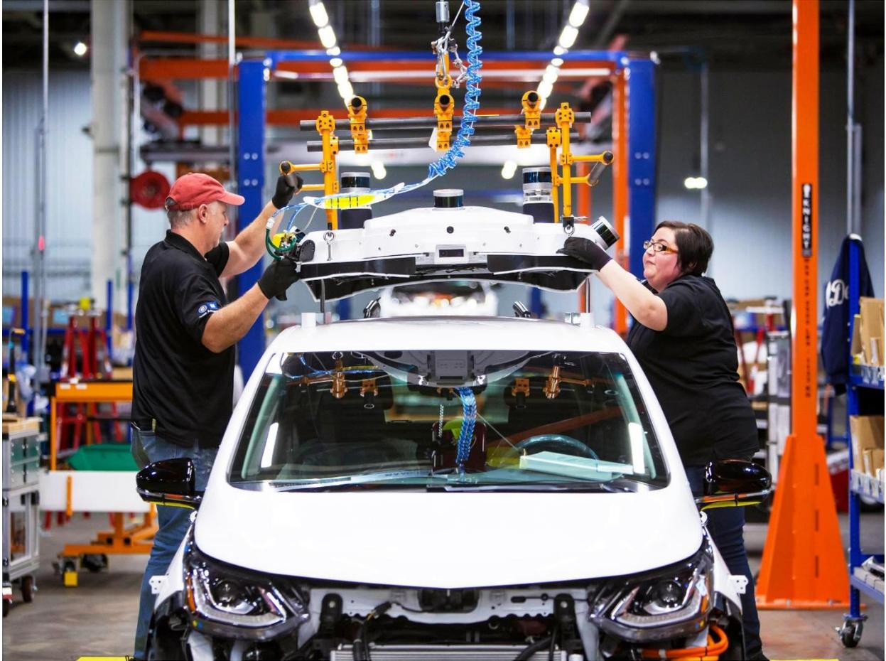
Workers at the Orion assembly plant adding the roof sensors for a Cruise self-driving car
