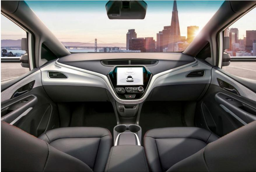
The inside of a level-4 self-driving car from Cruise.
