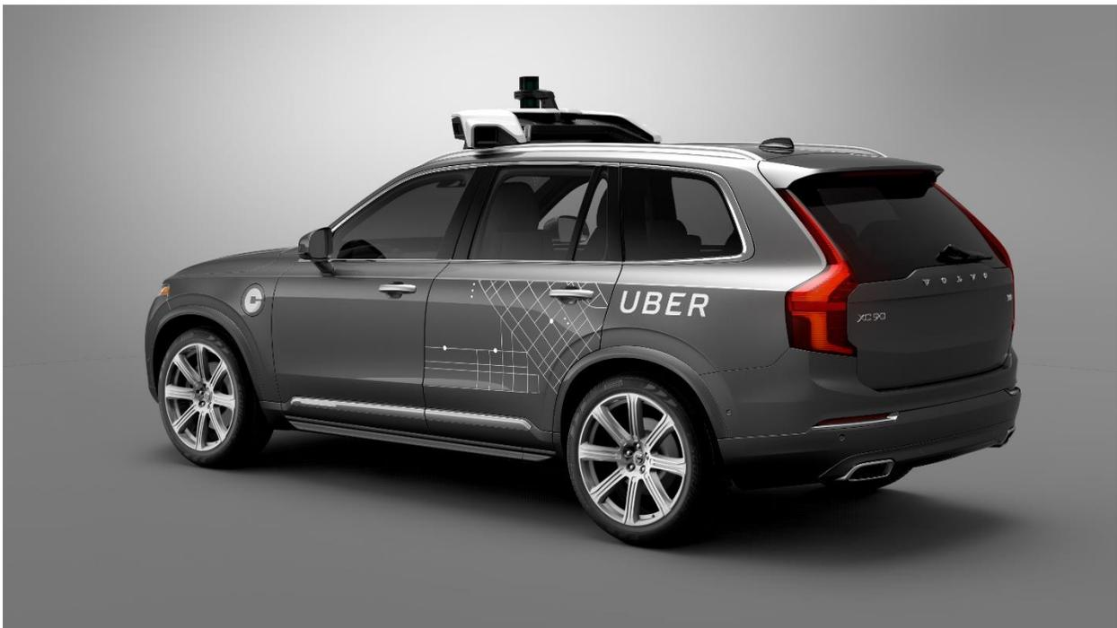
An Uber self-driving car based on a Volvo XC90
