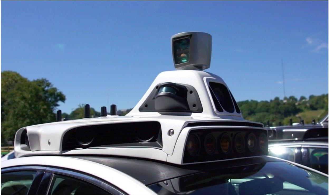
Older Uber Lidar sensor rack (Ford Fusion)
