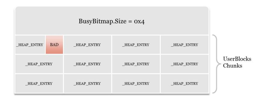
By making the PreviousSize of a chunk header to free larger than BusyBitmap.Size, an attacker can NULL out bits.
